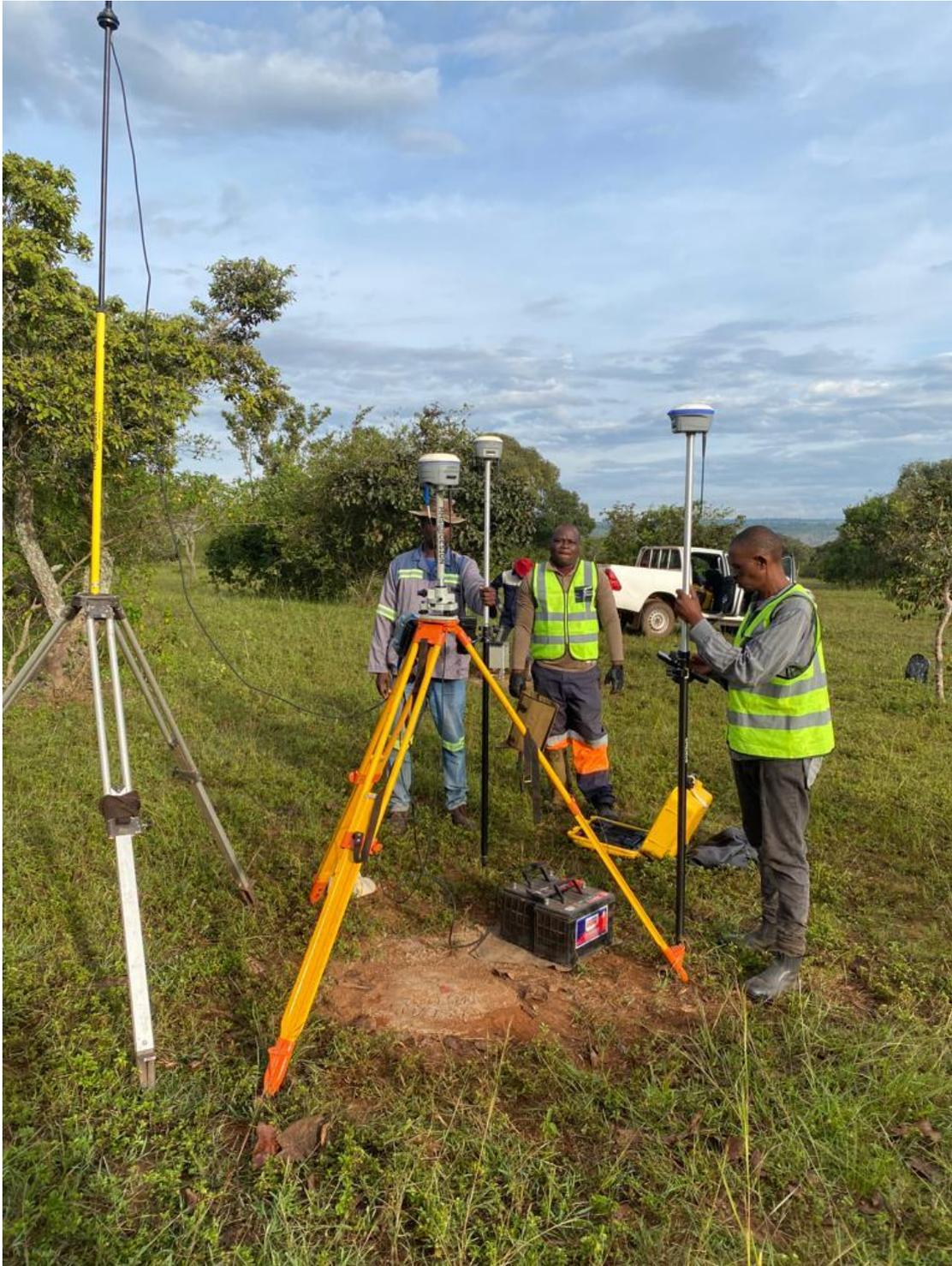
*Pictures: Setup and calibration of gravity survey equipment by exploration team at Kabanga Jirani NE Licences.*
