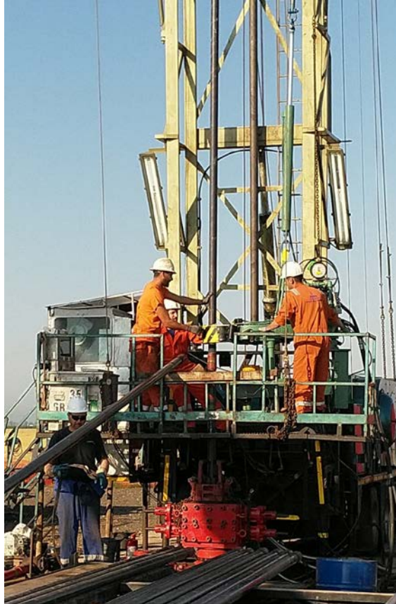
Running production string into IMIC-1 well prior to perforation
