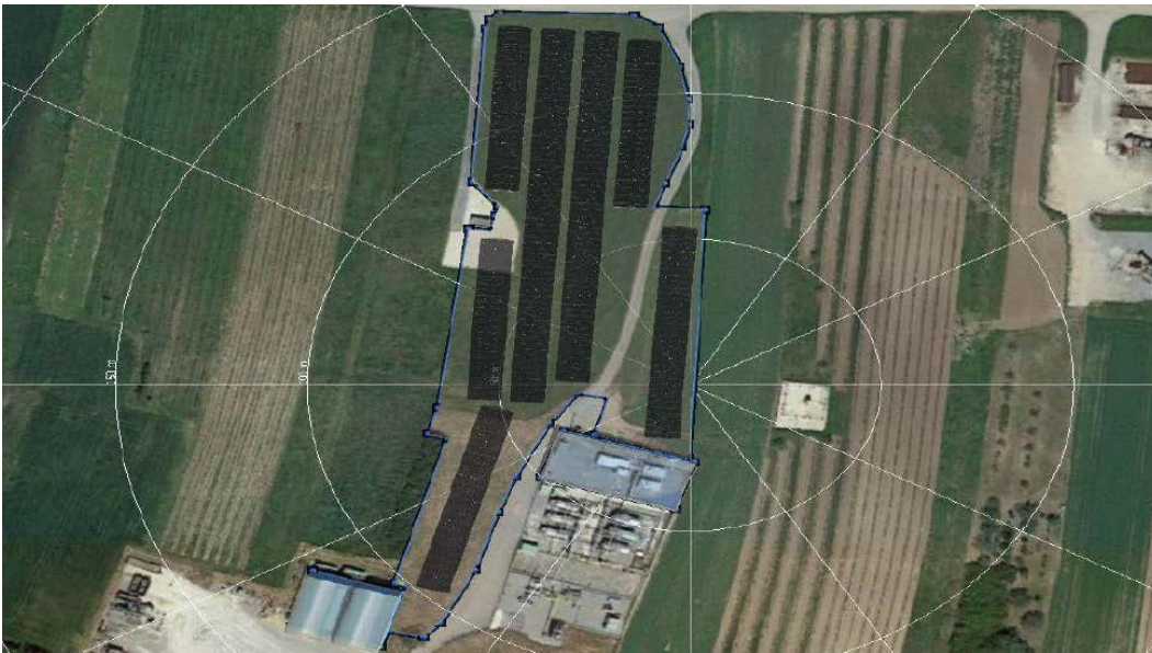
Figure 5: Potential layout of the PV panels at the Gaiselberg site (approx. 1 MWp)
