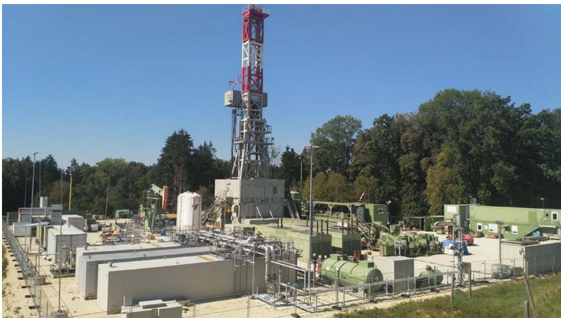
Figure 2: Shows the RED E-202 rig drilling the ANS-2A well at the Anshof PPF location in the ADX-AT-II exploration licence. On the left hand side of the rig the rod pump on the Anshof-3 discovery well can be seen
