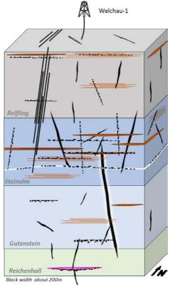
Figure 4: Welchau Carbonates Conceptual Model of an Open Permeable Fracture Network and other transmissibility events seen in the well such as reactivated beddings
