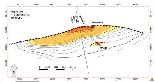
Figure 3: Welchau-1 Top Steinalm Formation post drill map. The 1989 MolIn-1 gas discovery is interpreted as a separate accumulation that is not connected to Welchau-1
