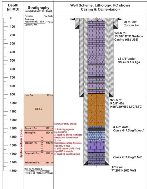
Figure 1: Welchau-1 casing schematic, stratigraphy and hydrocarbon shows encountered while drilling
