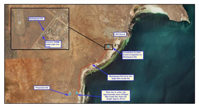
Figure 9. Conceptual location of new water supply pipeline
