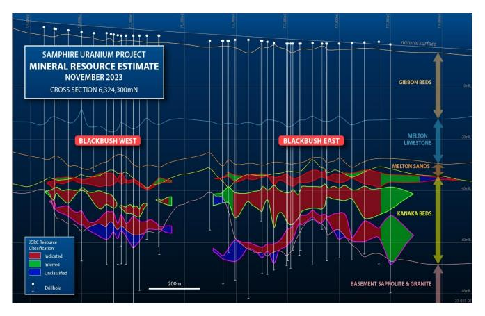
**Figure 7**: Mineral Resource classification, Blackbush west to east section 6,324,300mN (view looking north) showing four levels<sup>18</sup> of sub-horizontal uranium mineralisation. Note: the orientation of the cross-section cuts through generally perpendicular to the orientation of uranium mineralisation at Blackbush West and parallel (longitudinally) to orientation of uranium mineralisation at Blackbush Kest and parallel (image courtesy of AMC Consultants).
