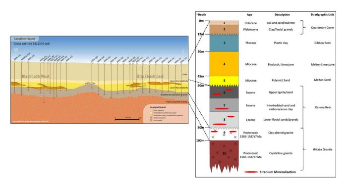
**Figure 3**: Cross section 6324300 mN through the Blackbush Deposit (15x vertical exaggeration, depth in RL metres) showing multi-level zones on simplified geology. Cross section constructed from pU3O8 intersections from AGE sonic core hole BBRM22-034<sup>9</sup> and historic drilling  $eU_3O_8$  intersections<sup>10</sup>. Detailed *s*tratigraphic section (modified after USA Internal Report, 2012).
