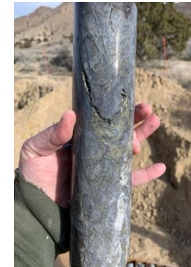
7DD21-003 @ 488m: Strongly altered diorite and porphyry; 7-10% sulphides with pyrite>molybdenite
