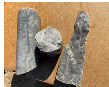
7DD21-003 @ 45m: Porphyry with extensive silica and potassic alteration; 2-4% sulphides pyrite>molybdenite>chalcopyrite
