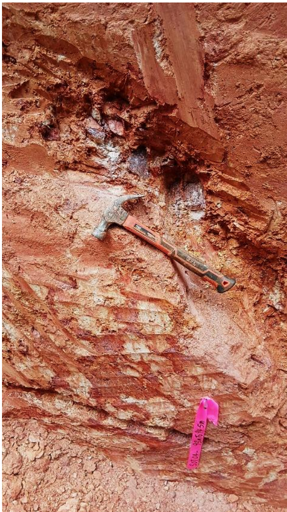
Figure 6: Presence of weathered quartz carbonate and sulphides within Trench 4 (93 – 94.5meters), Line 696000N. The Company is not implying any possibility of gold mineralisation or any other commercial metal, and this image is to provide general commentary on geological composition within South Oko which demonstrates geological continuity of the Barama-Mazaruni Greenstone from neighbours. This image and references to this image does not imply mineral abundance or pertain to a visual estimate of mineralisation. Figure 6 is evidence of general wall-rock geological observations made, which consist of weathered carbonaceous sediments and mafic Barama-Mazaruni greenstone (sulphides), and not commentary or implication of mineralisation at any specific sample or spot.
