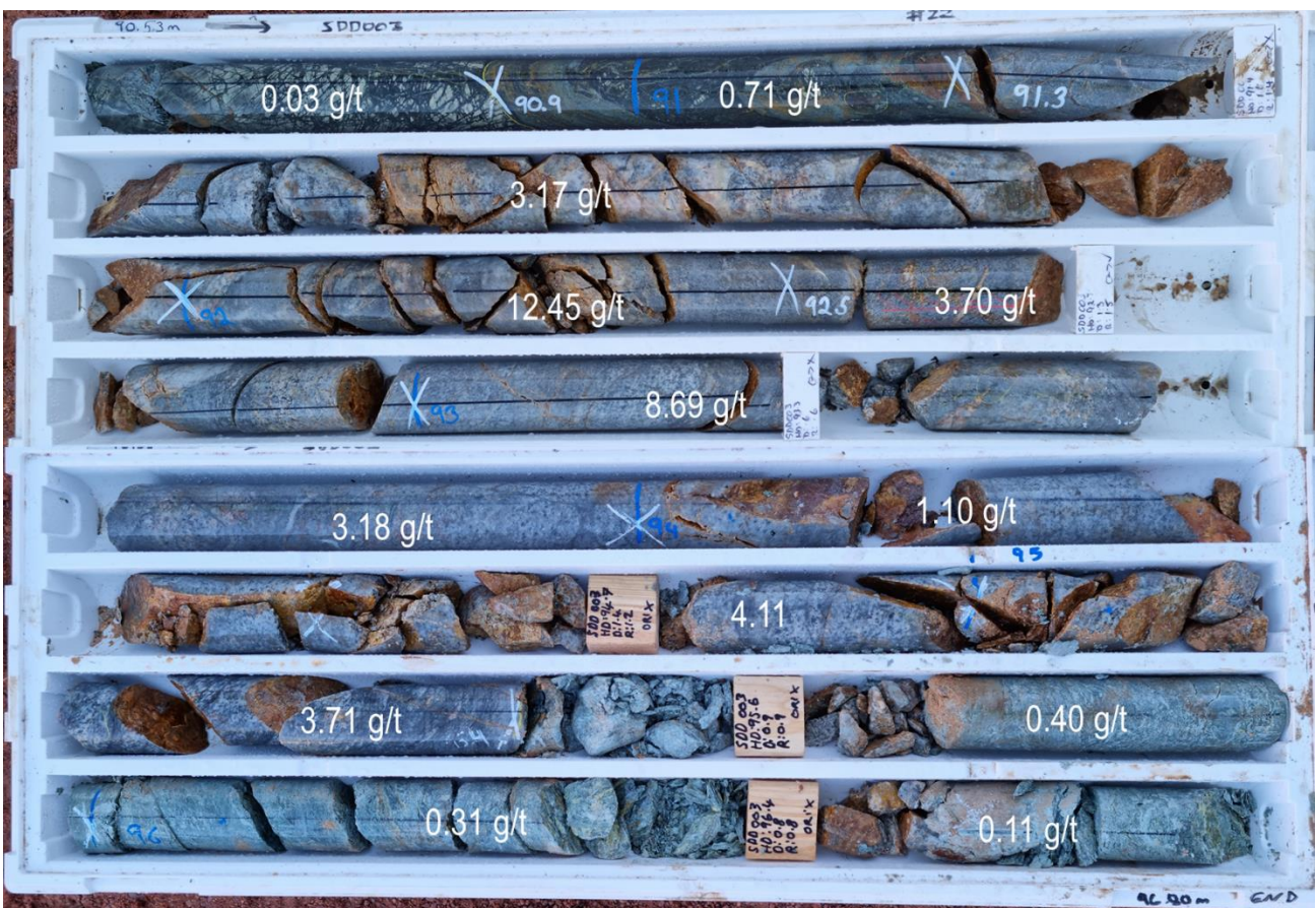
Figure 8: (SDD003) -Orion Lode HQ (63.5mm) diamond core from 90.53m to 96.8m showing high-grade gold mineralisation in pyrite-quartz veining, along the contact between silicified granodiorite and strong foliated ultramafic contact
