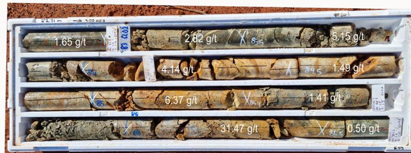
Orion Lode HQ3 (63.5mm) diamond core from 82.71m to 86.7m showing high-grade gold mineralisation in oxide and transitional zone. SDD008.
