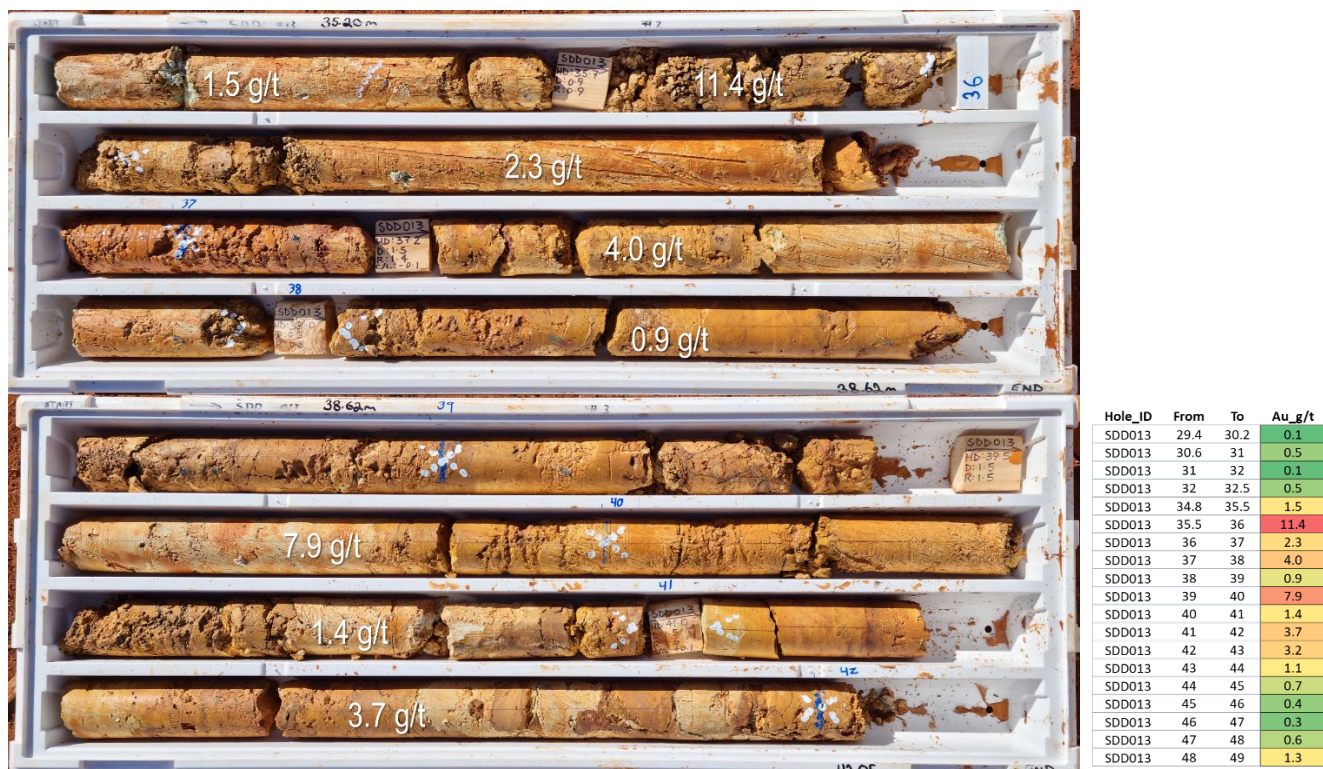
Figure 21. Diamond core from SDD013 from 35.20m to 42.05m HQ (63mm diameter). (Table to the right) Summary assay table for SDD013 from 29.4m to 49m
