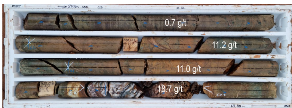
Figure 20. Diamond core from SDD016 from 59.05m to 62.5m HQ (63mm diameter). (Table to the right) Summary assay table for SDD016 from 59m to 66m
