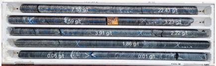
Lord Nelon NQ (47.6mm) diamond core from 213.42m to 222.58m showing high-grade gold mineralisation in strong quartz-pyrite veining, along the contact between silicified granodiorite and strong foliated ultramafic contact. SDD008
