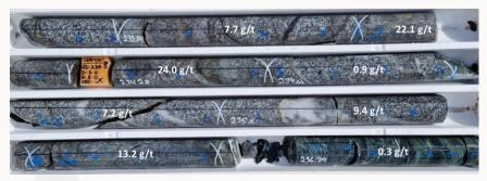
Lord Nelson HQ3 (63.5mm) diamond core 233.2m to 236.8m showing strong sulphide rich alteration. SDD001.
