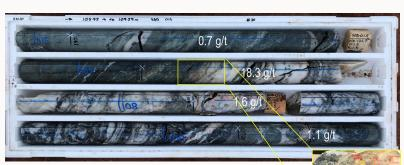
Figure A. Diamond core from SDD015 from 105.95m to 109.59m with visible gold at 107.4m in HQ (63mm diameter). SDD0015 intersected a quartz-rich laminated shear vein from 107.3m to 109.2m, within a broad 28m wide zone of extensional quartz veins, with distinct haloes of coarse-grained pyrite, from 88.5m to 116.5m, Overall intercept assayed 30m @ 3.0 g/t gold, incl. 1m @ 18.3 g/t gold from 107m
