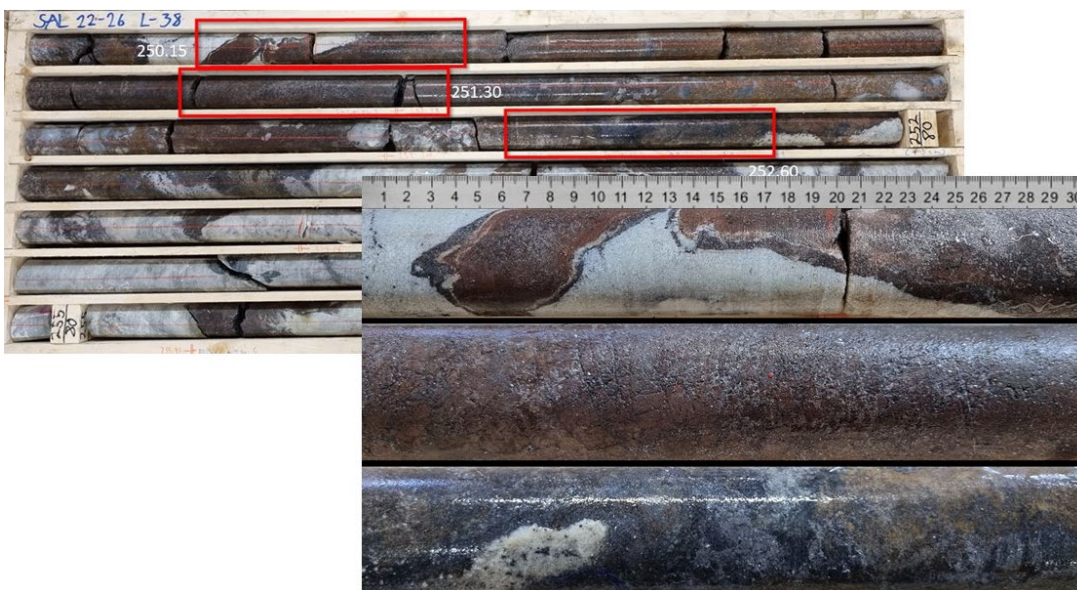
Figure 1: Massive sulphides intersected in Drillhole SAL2226
