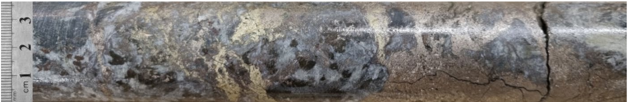
Photo 4: Sphalerite dominated mineralisation at 402.75m.
