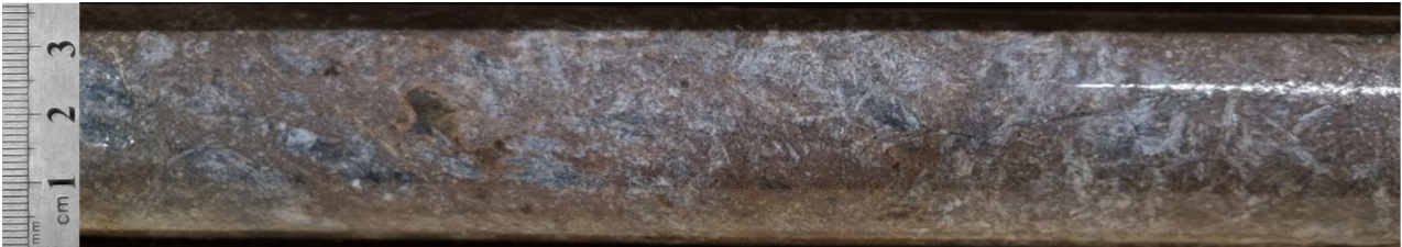
Photo 5: Massive sulphide with sphalerite >> galena-chalcopryite-pyrite-pyrrhotite mineralisation at 523.75m.
