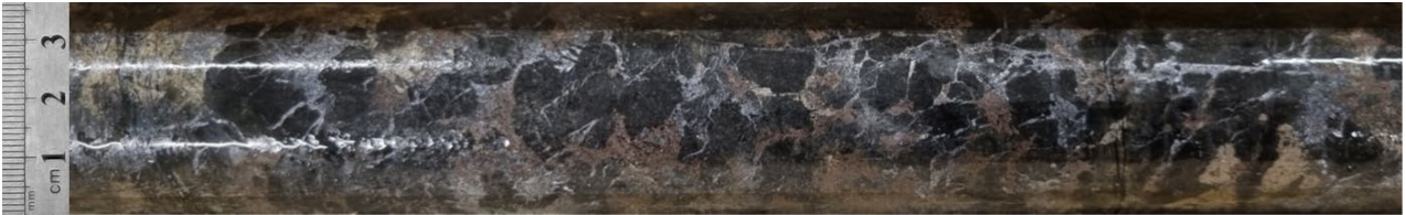
Photo 3: Pyrrhotite-chalcopryite mineralisation at 389.75 meters.
