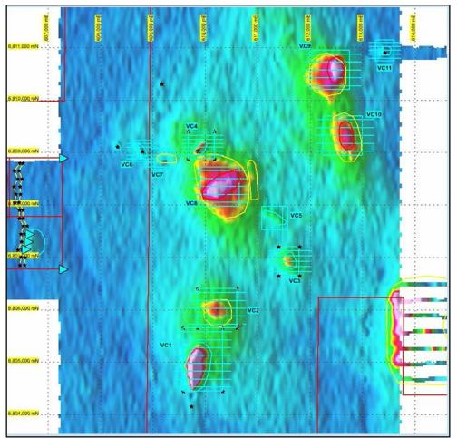
Figure 7. 2020 plan showing FTEM survey positions overlying high-interest targets from VTEM survey results
