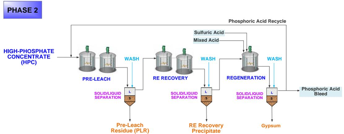
Figure 1: Phosphate Extraction Circuit
