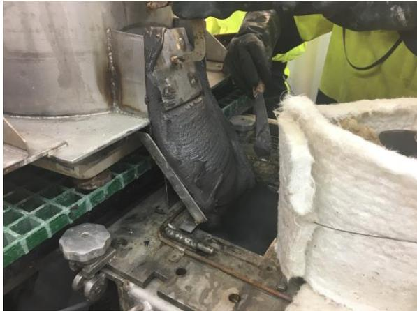
**Mixing During Acid Bake Showing Visible Paddles**
