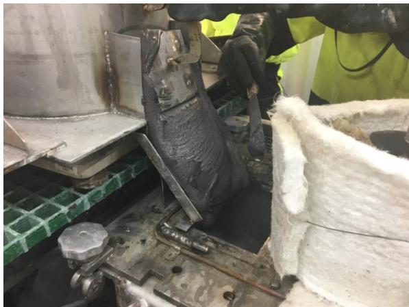
Mixing During Acid Bake Showing Visible Paddles
