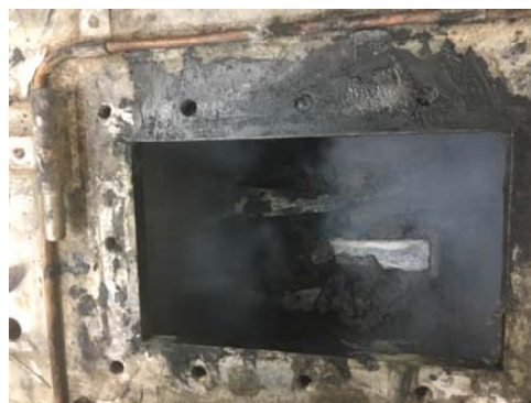
Mixing during Acid Bake showing visible Paddles
