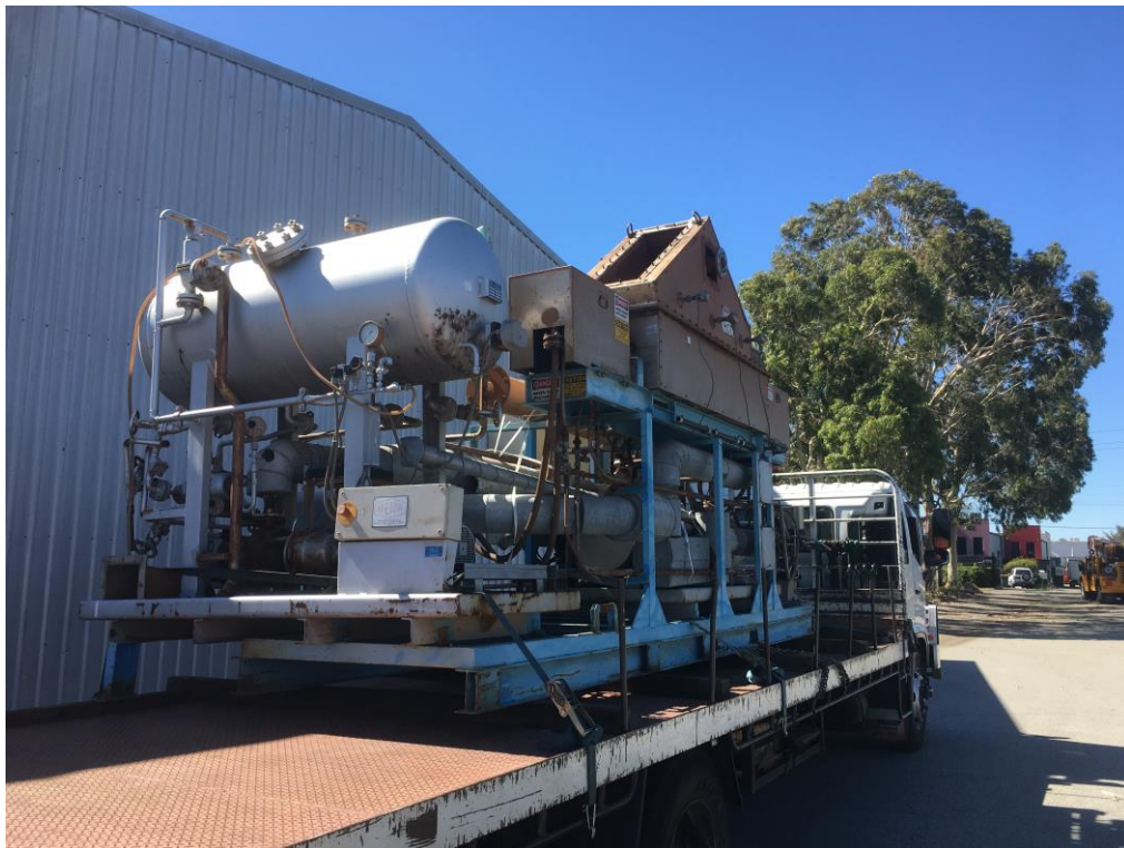
Paddle dryer pilot skid with oil heater
