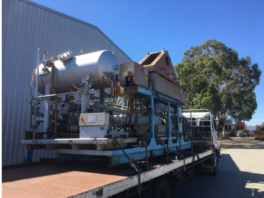
Image 1: Paddle dryer pilot skid with oil heater
