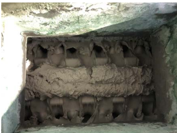
Figure 3: Komline paddle dryer in operation
