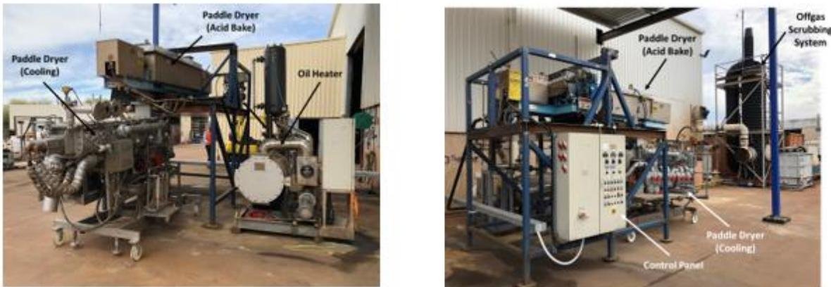
**Figure 4: Sulphated Nolan's material being cooled in Gouda (L) and discharging (R)**
