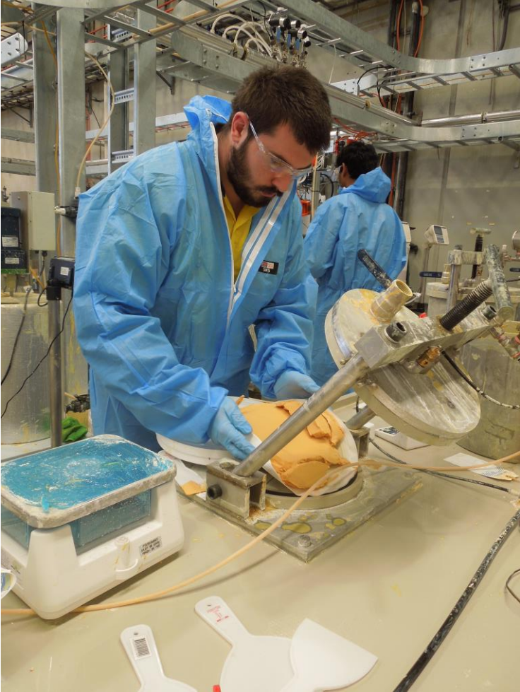
Refined NdPr-rich Rare Earth Hydroxide Precipitate being removed from filter unit
