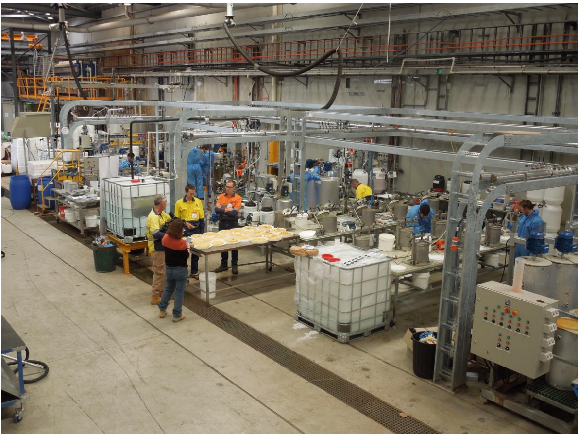
Phase 5 Rare Earth Purification and Precipitation Pilot Plant
