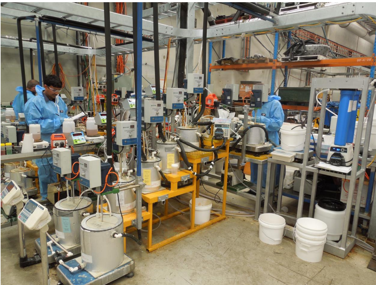
Phase 6 Pilot Plant: Rare Earth Hydroxide Dissolution Circuit
