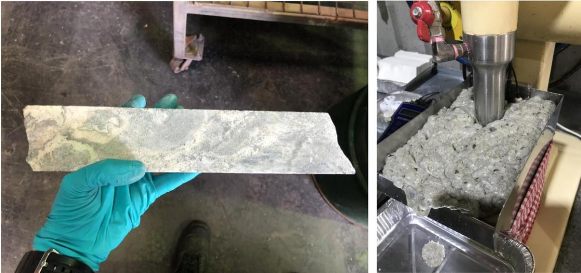
**Figure 1: 5A2 drill core sample for flotation variability program (left) and flotation test (right).**
