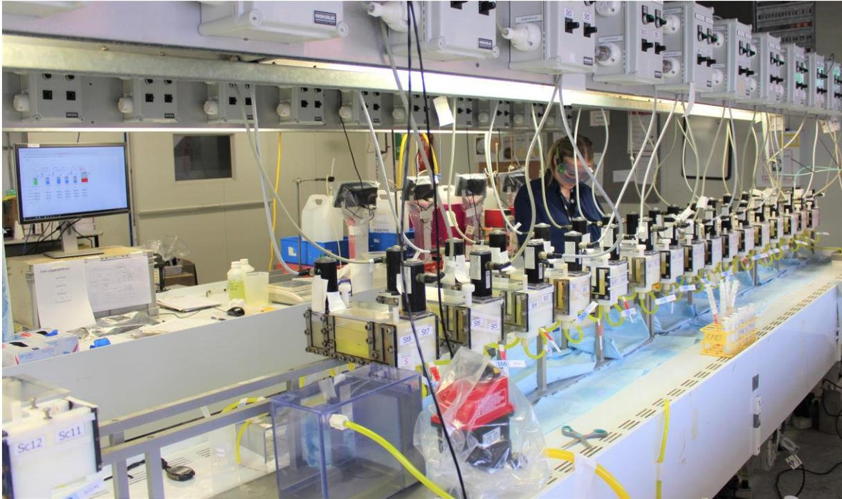
**Figure 2: SEG-HRE separation circuit during pilot operation at ANSTO in December 2019**
