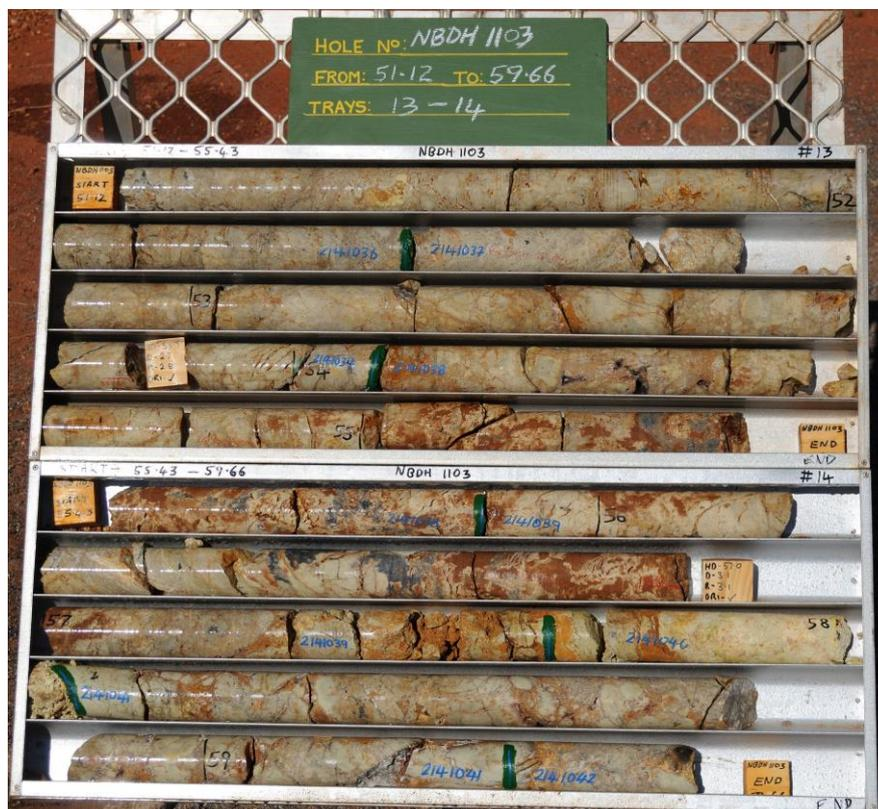
**Figure 4: NdPr-rich apatite intersection (51.12m – 59.66m) in drill core from hole NBDH1103.**
