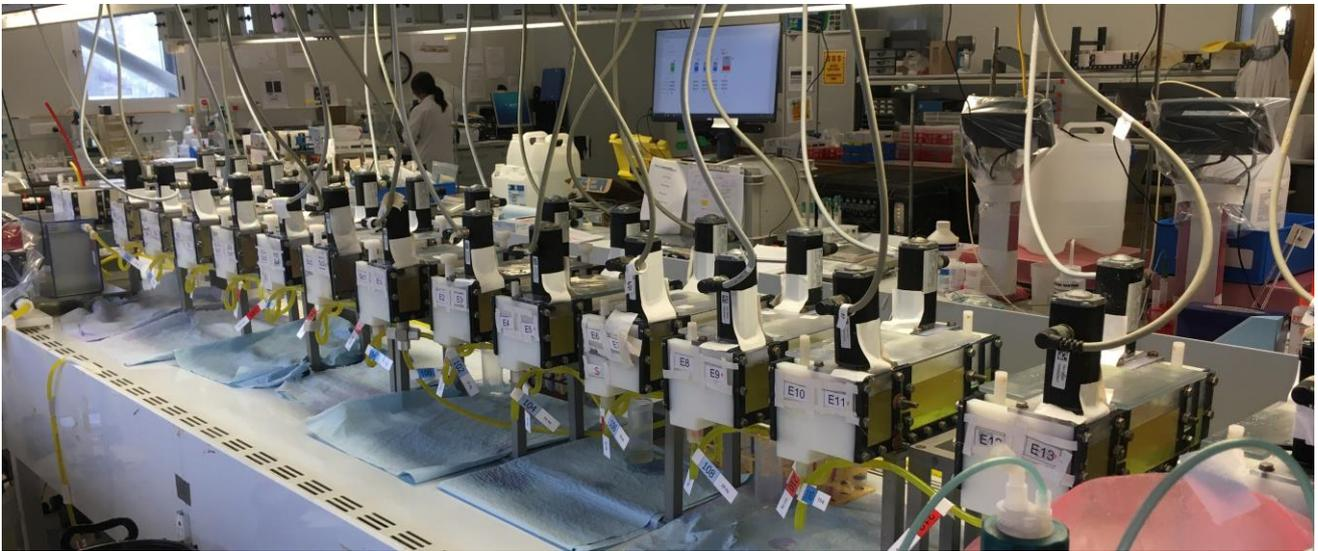
Figure 2: Side on view of SX mixer-settlers in the NdPr separation circuit during pilot operation
