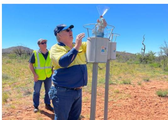
Figure 3: Passive dust collection monitoring
