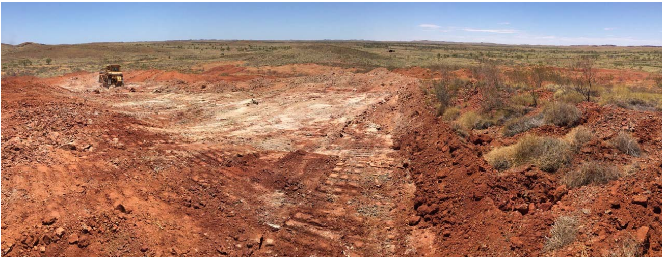
Figure 2. Artemis, Silica Hills Project – Karratha. Bulldozer costean exposing multiple quartz veining in felsic and mafic rocks.
