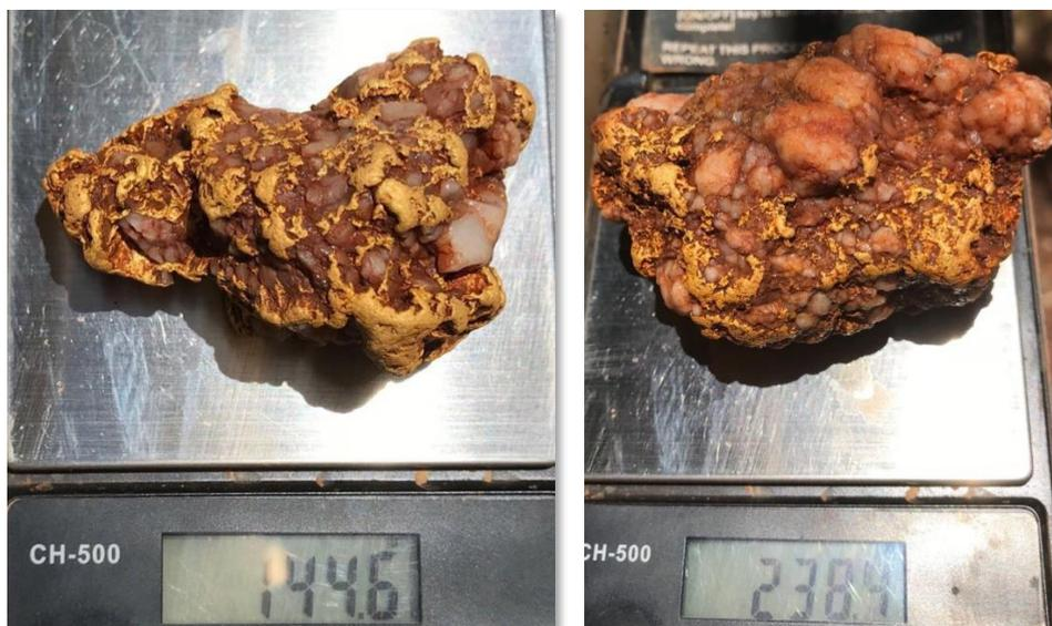
Figure 1: A sample of specimen quartz/gold nuggets recovered Friday 24<sup>th</sup> November from oxidised rock above primary quartz veins and stock work. 144.6grams (4.6oz) and 238.4 grams (7.7oz).
