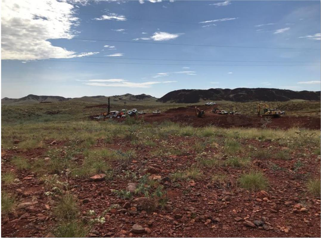
**(Figure 1: Photograph of the Powerline showing looking southeast. Trenches are being opened immediately right of the location of the diamond core rig. The base of the conglomerate sequence is in the foreground and the top is approximately where the two white vehicles are parked along the ridgeline. True thickness of the conglomerate section is approximately 30 meters and is dipping away from the camera at about 3-4 degrees.)**
