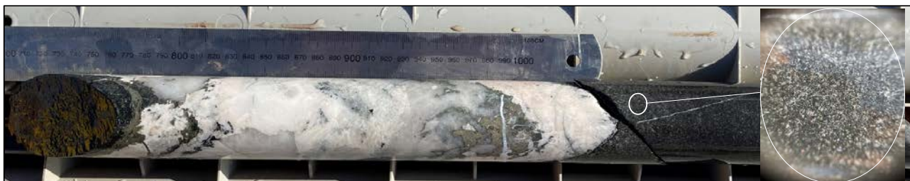
Figure :3 GDRCD007 - 538m, example of quartz-calcite vein in altered diorite with abundant pyrite± chalcopyrite-chlorite-actinolite infill. Close up example of disseminated inter-matrix sulphides in altered diorite.
