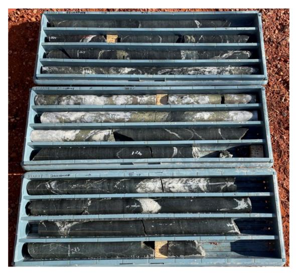
Figure 12: 22CCRD008 (263-273.5m) lower interval of significant vein hosted sulphide forming part of the broader 16.6m interval with a significant grade of 3.14m @ 6.38% Cu, 3.61% Cu, 0.059% Co from 265.92m
