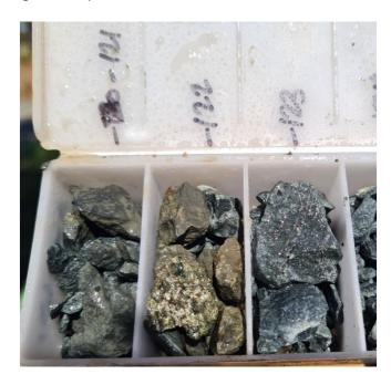
Figure 28: Mineralisation occurrence in ARC401 showing some 'massive' style of sulphides
