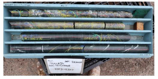
Figure 11: Part of the upper zone of the broader 16.6m showing the massive sulphide interval with brecciated upper contact which returned a result of 1.18m @ 15.65% Cu, 5.40g/t Au, 0.090% Co from 256.84m.
