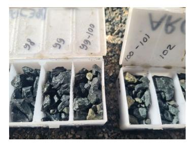
Figure 27: Sulphide mineralisation in Hole ARC398 from 99 to 103m
