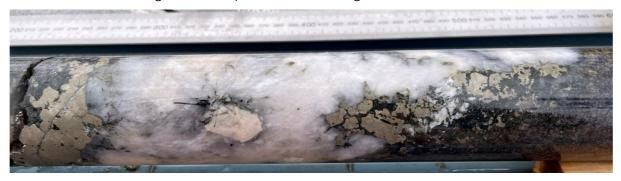
Figure 5: GDRCD007 - 547m, example of a large quartz calcite vein in altered diorite with semi-massive sulphides pyrite +/-chalcopyrite as well as chlorite actinolite infill and alteration halo.
