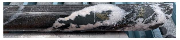
Figure 6: GDRCD007 - 559m, example of a quartz qalcite vein in altered diorite with pyrite +/- chalcopyrite, chlorite 'jigsaw' infill
