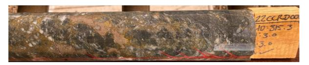
Figure 13: 22CCRD008 mineralisation occurrence at EOH 315.3m.
