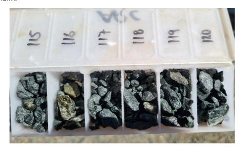
Figure 17: Sulphide occurrence in ARC403 comprising pyrite and pyrrhotite.
