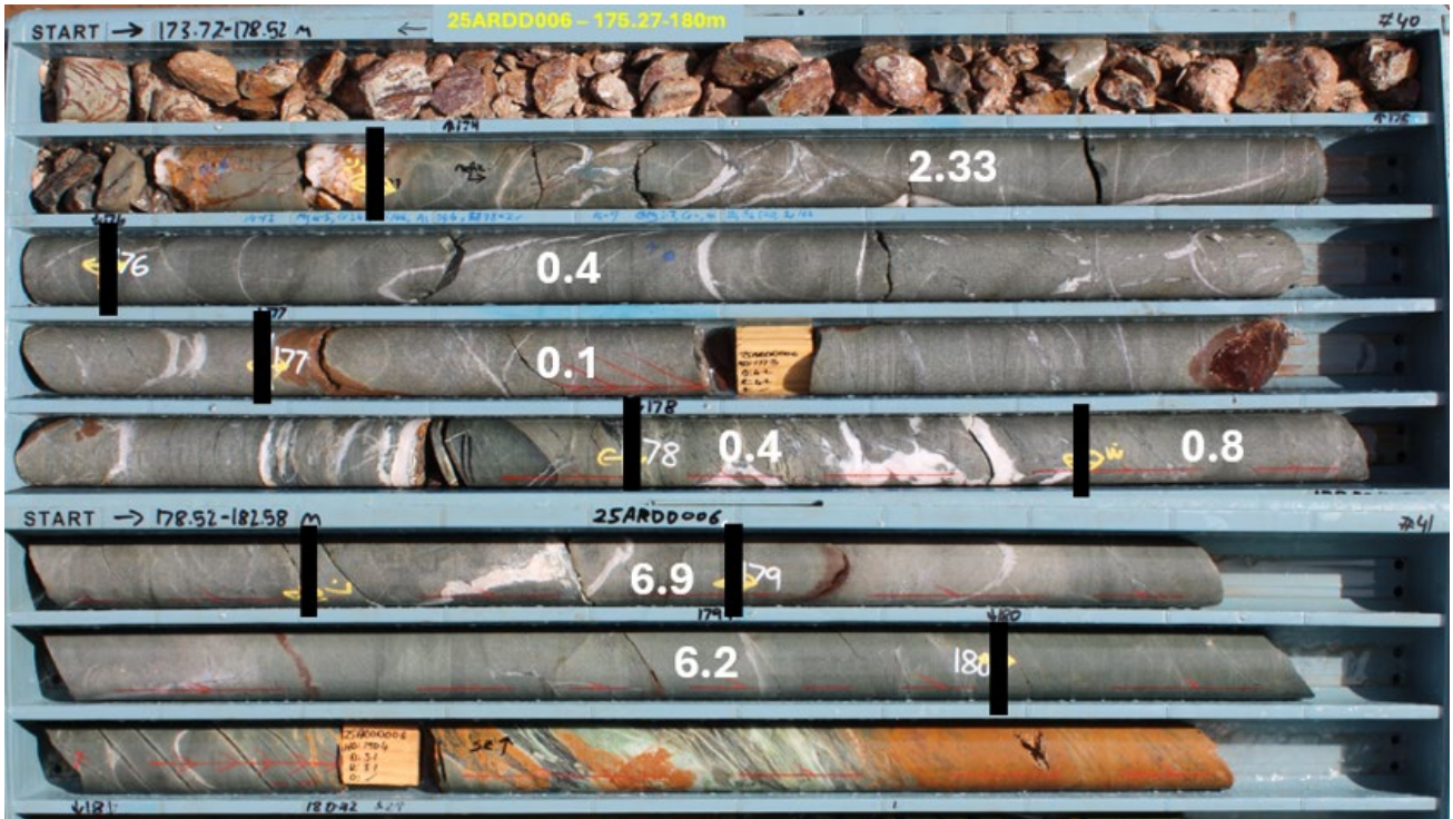
Figure 1 – 25ARDD006 173.72m – 178.52m core including Au g/t results over significant intercept see Table 1.
