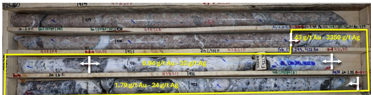
Figure 10. Diamond hole CBD243 Delia SE quartz breccia intercept, 2.0m @ 1,507g/t AgEq from 420.5m to 422.5m. Refer to Andean ASX release dated 11 December 2025.
