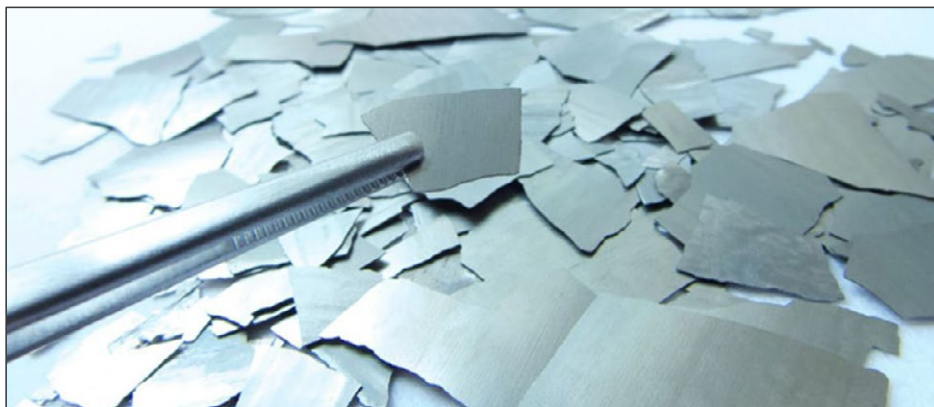
Figure 3.4: Example of finished NdFeB strip alloy product
