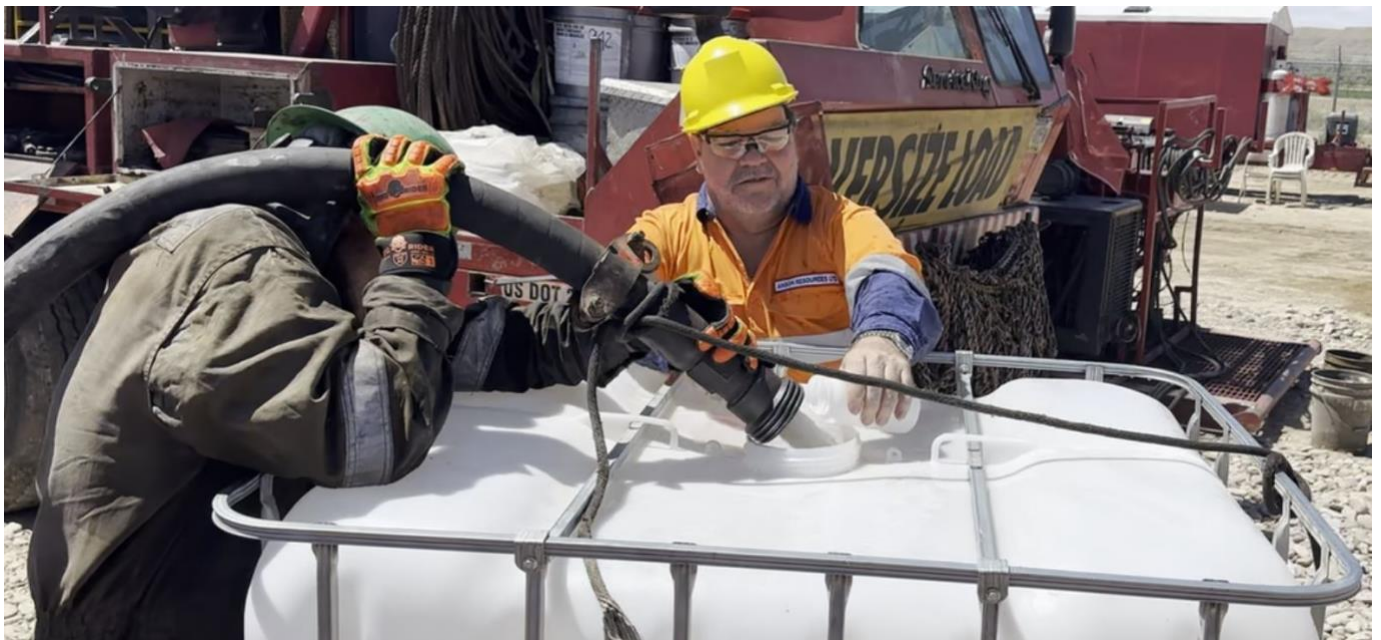
Figure 1: Sampling the brine from the Leadville Formation, Mississippian Units at Bositydaba#1 well.
