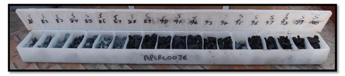
Photo 2: Chip tray from hole APSRC0038 depth 80-100m showing sulphides in a basaltic unit in each one metre interval. Note the colour changes from leucocratic depths 81-83, 86-87 and 95 to melanocratic phases and the 1% sulphide content at 98m.
