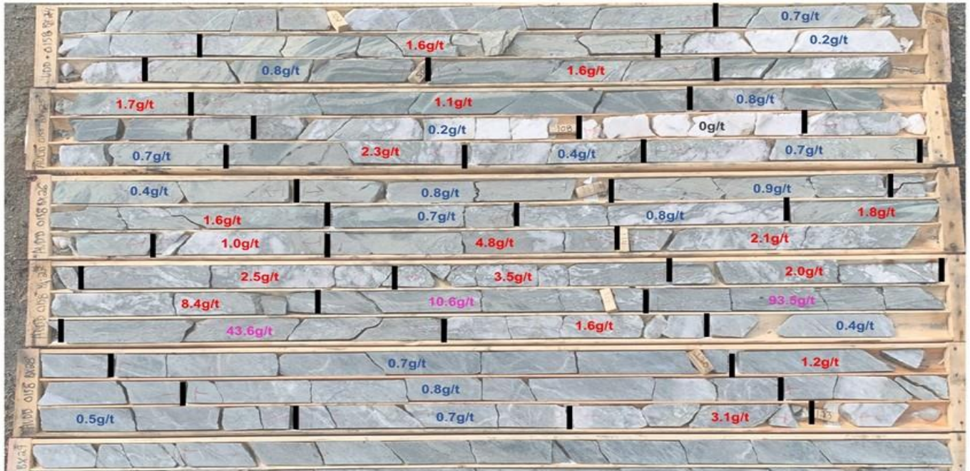
Figure 5: AUDD0158: New Discovery. 102.65m to 123m. Sericite-ankerite-pyrite altered intermediate dyke within sericite-ankeritepyrite altered Quartz-Feldspar-Porphyry. Alteration to the selvage of and is related to multiple sheared Quartz-Ankerite-Pyrite veins. Interval is 20.4m @ 5.3g/t Gold including 2.2m @ 39.3g/t Gold from 116m.
