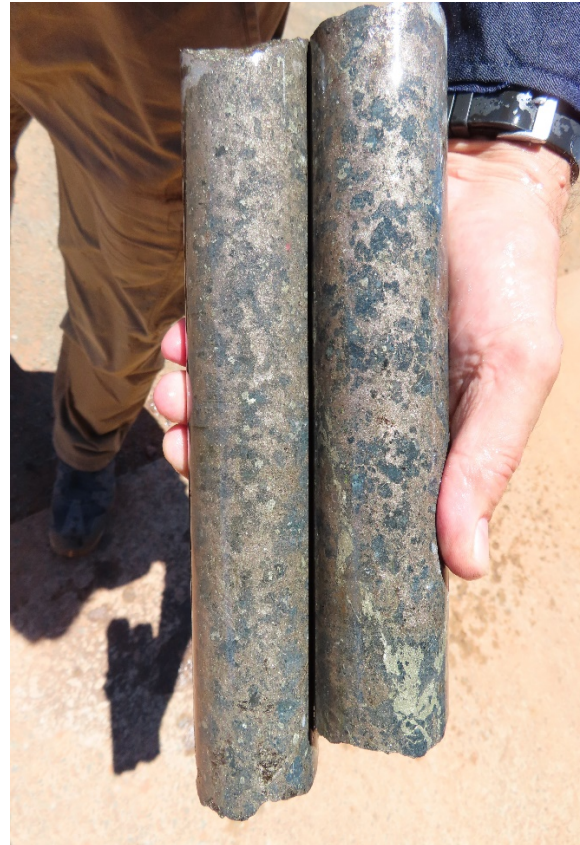
Figure 2: ANDD0004 drill core Matrix Ni-Cu sulphides @ 353.3m
