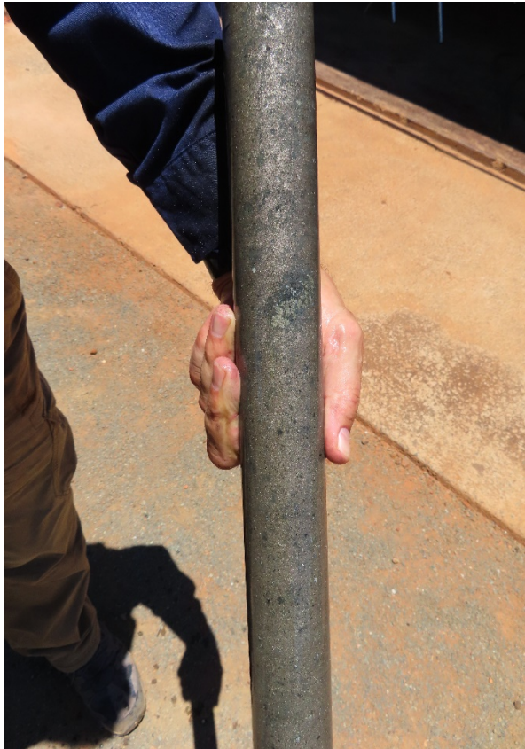
Figure 1: ANDD0004 drill core Massive Ni-Cu sulphides @ 357.5m
