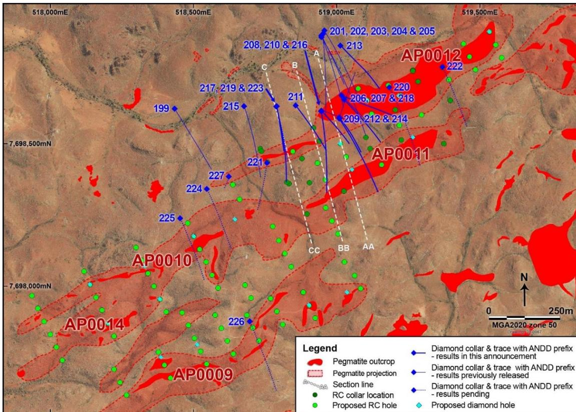
**Figure 2: Pegmatite outcrops, drilling and section lines at AP0011 / AP0012**
