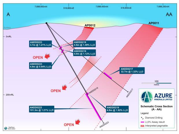
Figure 3: Section A-AA through AP0011 / AP0012 pegmatites with reported lithium intersections
