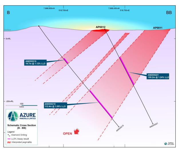
Figure 4: Section B-BB through AP0011 / AP0012 pegmatites with reported lithium intersections
