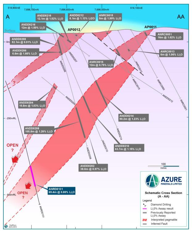
Figure 3: Section A-AA through AP0011 / AP0012 pegmatites with reported lithium intersections
