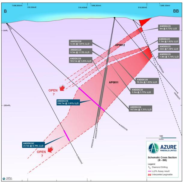
Figure 4: Section B-BB through AP0011 / AP0012 pegmatites with reported lithium intersections
