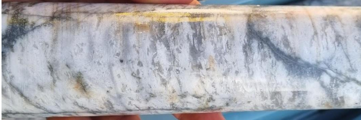
Figure 2: Photographs of visual fine to coarse-grained crystalline spodumene mineralisation in AP0003/AP0004 and AP0005 pegmatites at Target Area 3
