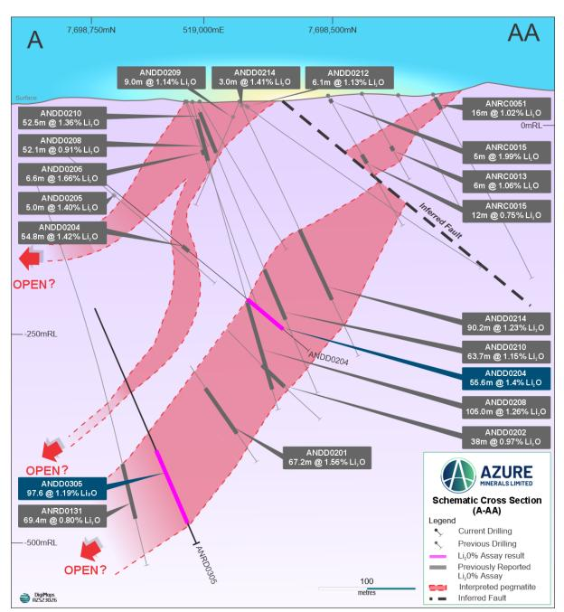
Figure 3: Section A-AA through AP0011 and AP0012 pegmatites with reported lithium intersections
