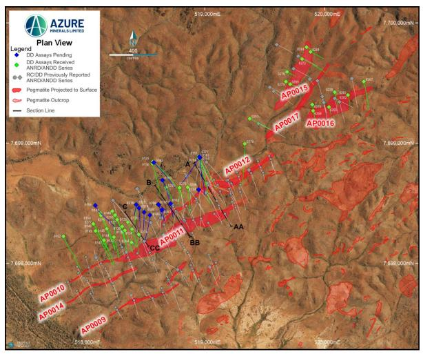
Figure 2: Pegmatite outcrops, drilling and section lines at the AP0011, AP0013, and AP0015/AP0016/AP0017 pegmatites
