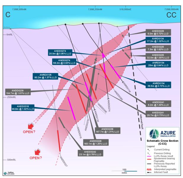
Figure 4: Section C-CC through AP0011 and AP0012 pegmatites with reported lithium intersections
