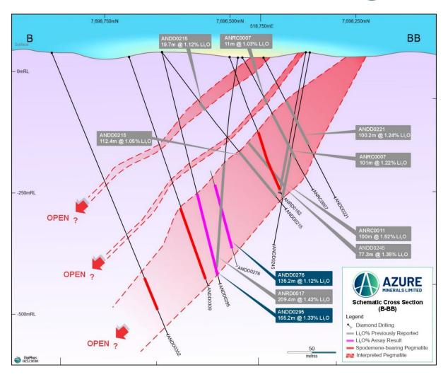
Figure 4: Section B-BB through AP0011 and AP0012 pegmatites with reported lithium intersections
