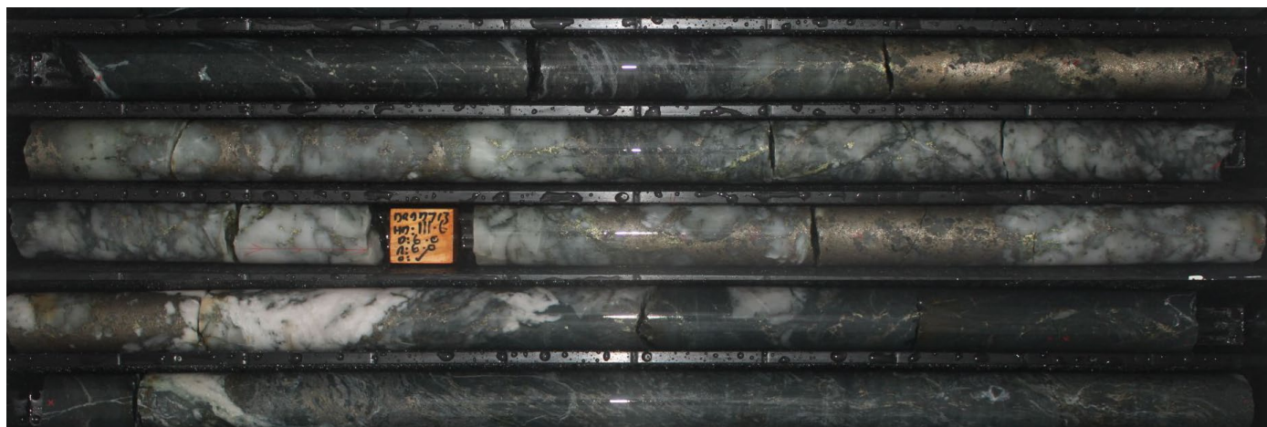
Figure 4: DRDD713 Tribune Grade Control diamond hole intersected as a large milky/smoky quartz vein with fracture fill pyrrhotite and chalcopyrite. 15+ flecks of visible gold observed , mostly forming around the cataclastic pyrrhotite. Strong shearing on the margins. Assays pending.
