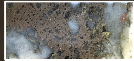
Close up of vein texture showing cataclastic quartz with well disseminated gold
