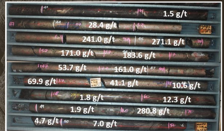
Recent grade control hole DRDD1545 10.8m @ 66.8 g/t from immediately below the 1018 level
