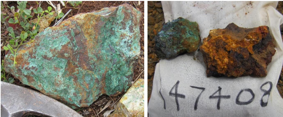
Photo 1. A (Left) - Mineralised subcrop at Flanagan's returned 5.1 % copper, 39 g/t silver 1.1 g/t gold (sample 147401). Photo 1B (Right) - rock chip sample 147408 assayed 9.8 g/t gold, 179 g/t silver and 12.1 % copper from old workings at Great Blackall.
