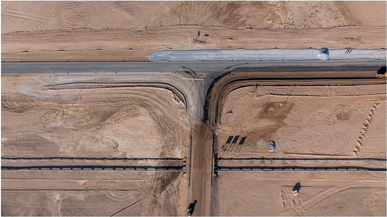
Figure 2: Widening of C28 intersection entrance area to improve safety as vehicles enter site access road
